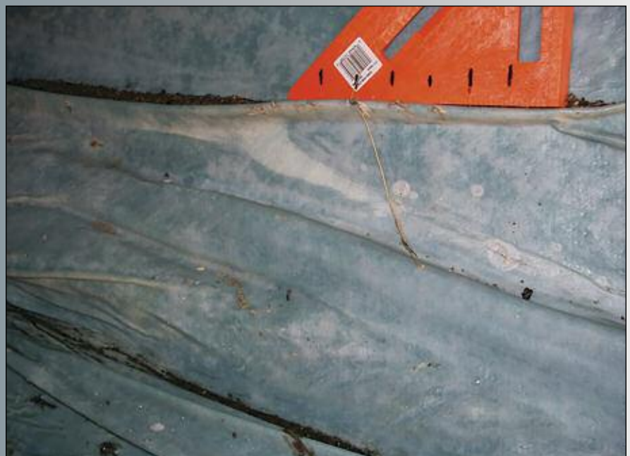
Figure 1. Significant WFF (wrinkles, fins and folds)
