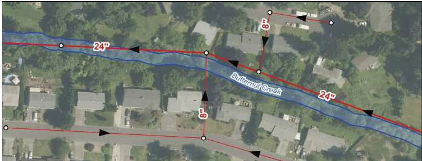
Figure A: Interceptor in relationship to creek
