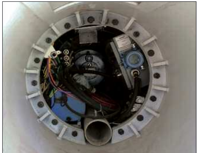
The compact SBU-RC operates using an in-shield drive motor for torque. View shows the inside of the SBU-RC with drive motor.
