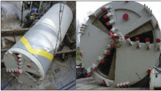
Figure 5. 60-inch Diameter Open Shield Pipe Jacking Machine Used on the Project
