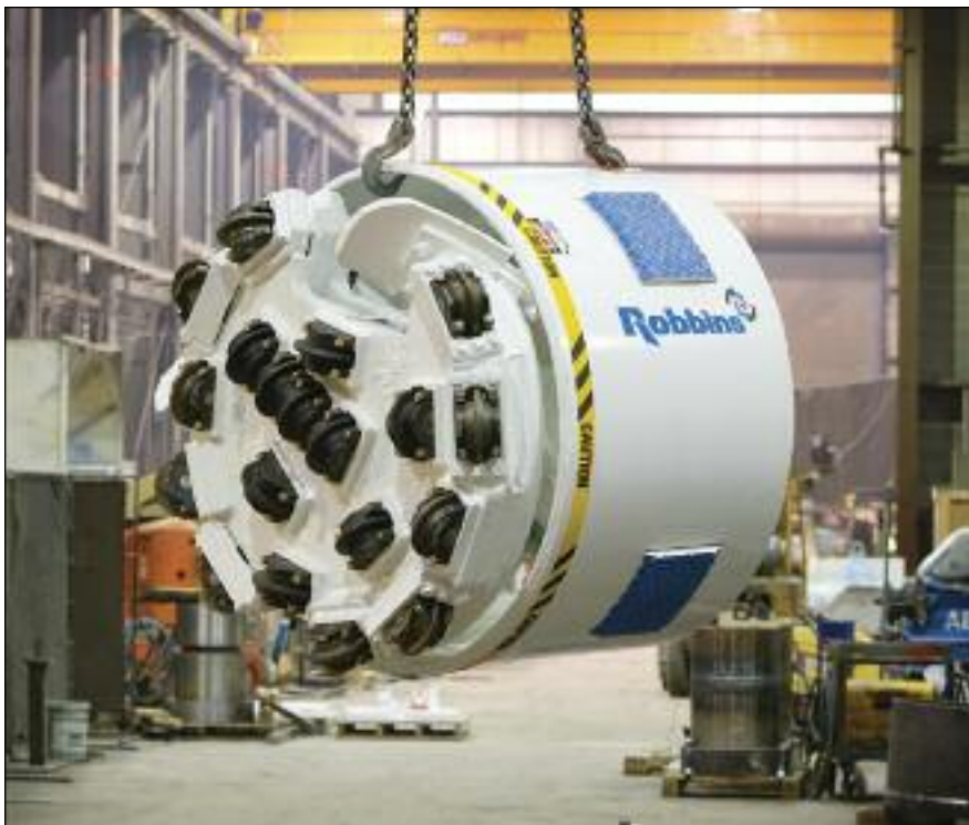
The Robbins Small Boring Unit (SBU-A) is capable of excavating mixed ground and hard rock up to 25,000 psi UCS.
