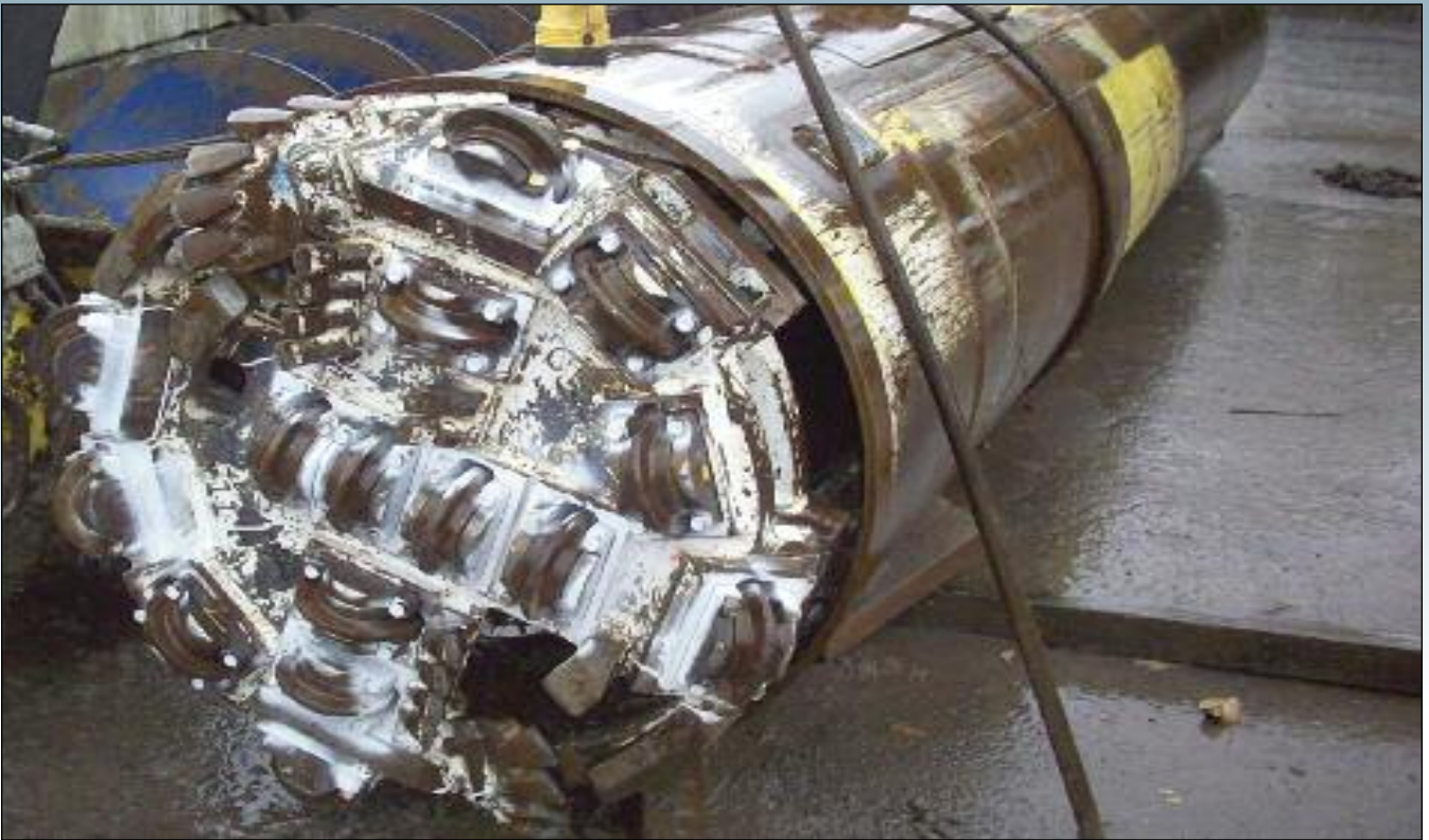
Completed in December 2009, the 600-foot bore in Tigard, Oregon, was a record for hard rock auger projects using disc cutters.
